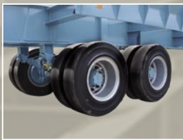
Pneumatic/Solid Rubber Tyres
