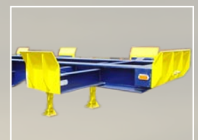
Guides for use with Fork Lifts
