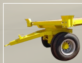
Heavy Duty Draw Bar with Towing Eye
