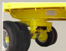
Heavy Duty Ball-Race Turn Table
